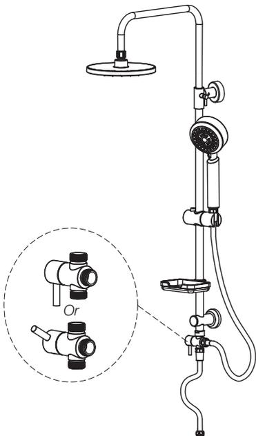
17. Regulate the water flow using the knob on the diverter.
