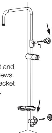
11. Undo the clamp on the upper wall bracket and adjust the length of the slide rail.
