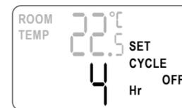
"CYCLE ON/OFF" will flash on the display to indicate that the program is active.
