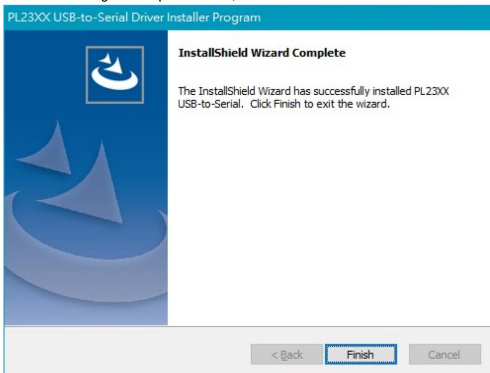
5. Plug in the USB to Serial adapter ( PL2303GC chip ) to the PC USB port. Windows should detect the driver as Prolific PL2303GC USB Serial COM Port. Go to Device Manager and check for the “Prolific PL2303GC USB Serial COM Port” device and the COM port number assigned by Windows.
