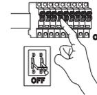
2. If necessary, remove the terminal block from the hanging loop and connect the incoming neutral wire (blue) to the terminal marked "N". Connect the live wire (usually brown) to the terminal marked "L".
